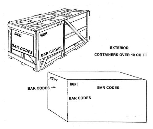
FIGURE 22. Exterior container bar code marking on boxes and crates 10 cubic feet and over.
