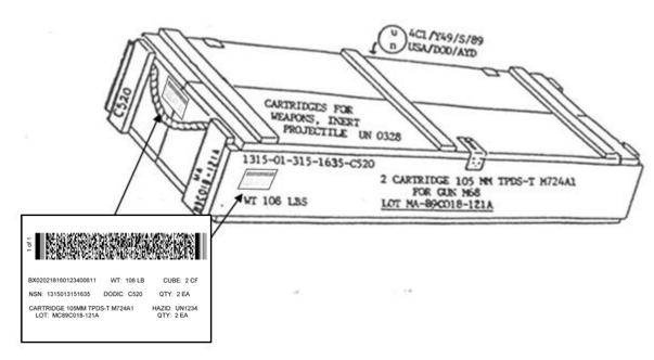
FIGURE 46. <u>Identification marking and the placement of ammo/explosives identification bar code labels on exterior rectangular containers.</u>
