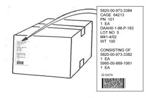
FIGURE 34. Single stock numbered item consisting of other stock numbered items in a single container.
