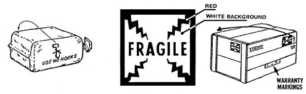
FIGURE 29. Examples of special marking (FRAGILE, UP, arrows, USE NO HOOKS and warranty marking).
