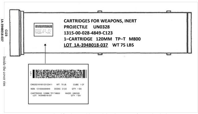
FIGURE 47. <u>Identification marking and the placement of ammo/explosives identification bar code labels for exterior cylindrical containers.</u>
