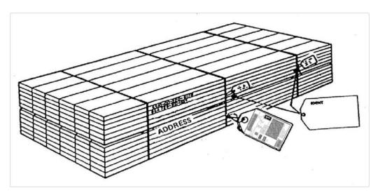
FIGURE 10. Placement of identification and address marking on bundled wood products.
