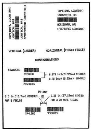
FIGURE 16A. <u>Linear (Code 39) bar</u> code configurations.
