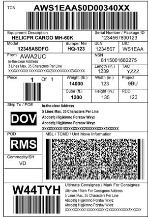
NOTE: Not actual size. Recommended label size is 4 by 6 inches (10.2 by 15. 2 cm). FIGURE 2A. Generic MSL. FIGURE 2B. Unit move MSL.
