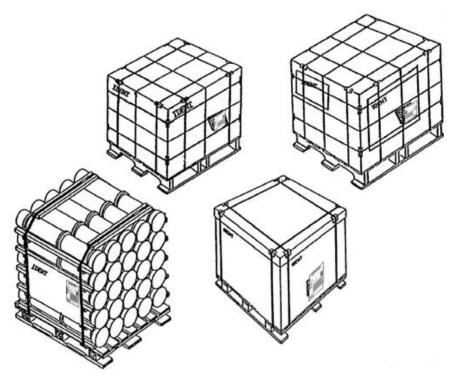
NOTE: For identification bar code specific marking locations, see Figure 25. FIGURE 9. Placement of identification and address marking on palletized unit loads.
