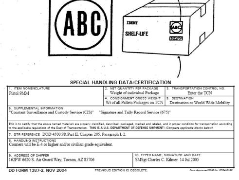
FIGURE 28. Examples of special marking (shelf life, project code, and transportation special handling/protective services marking).
