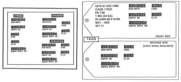
FIGURE 19. <u>Typical linear (Code 39) bar code configurations for use</u> on exterior containers and on tags.
