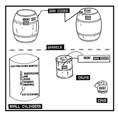
FIGURE 24. Bar code marking on cylindrical containers.
