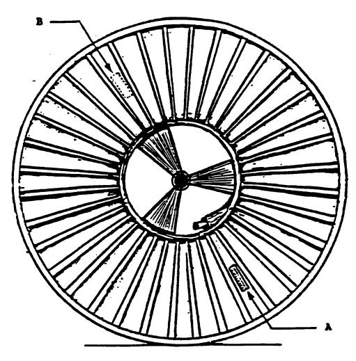
A = One Label should be placed adjacent to the cable starting hole.
