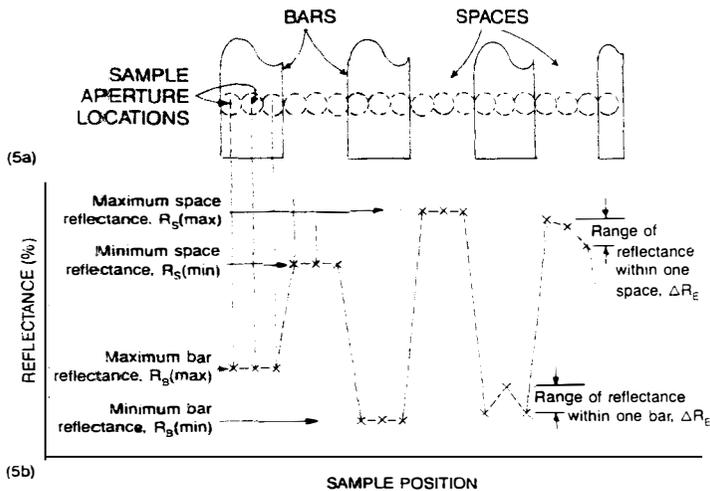
Figure 5. Bar Code Reflectance Measurements
